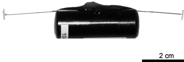
APPENDIX 1. – Image of 1 telemetry transmitter showing the T-tags glued by epoxy resin, ready for being inserted to a fish. Transmitters for L. bergylta and D. labrax had a third anchor point (see the text in materials and methods section for further details).
